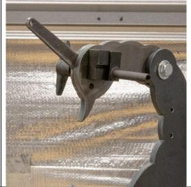
Step 13 Install the M10 Nut on the T handle thread, then install the tracking adjuster T handle until it contacts the back of the hinge.
