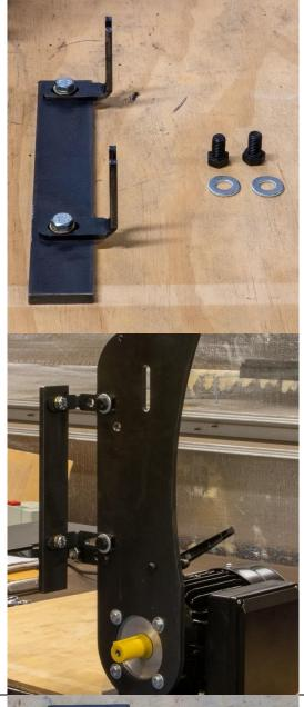
Step 10 Next assemble the work rest to the tool arm using 1 x M12\*35mm bolt and washer and 1 locking handle with a washer.
