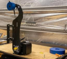
Step 17 Once the wheel is seated on the shaft, secure with the bolt, tighten to 20ft/lb. Step 18 Locate the supplied belt and hang it over the top wheel. Pull down on the tensioner handle to hook it under the drive wheel. Pay attention to the belt orientation, some can only be used in one direction.
